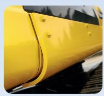
Extra heavy-duty, wraparound-type side protection (5/8"; 15 mm) bolted to each side of the upper structure to help secure your vehicle from debris or side impact.
