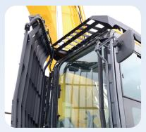
Prioritize safety with a cab that is ROPS compliant with ISO 12117-2:2008. Easy access for window cleaning with the hinged front guard.
