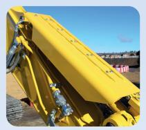
Stay resilient against the stresses of demanding environments with an attachment/bucket cylinder guard, reinforced bucket linkage and a heavy-duty boom lamp.
