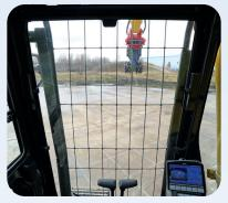
The one-piece front screen is fitted with high-impact protective glass to help shield debris and features a carefully aligned grid layout to minimize obstruction.
