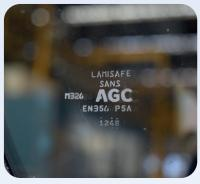
The front and roof windows are high-impact protective glass compliant with EN356 grade P5A. A wash/wipe system keeps the roof window clean for optimal visibility.
