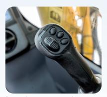
Get smooth, precise movement of your attachments with a joystick that features proportional control buttons for enhanced performance.
